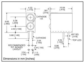
Standard Polarity shown in drawing: Cathode right
