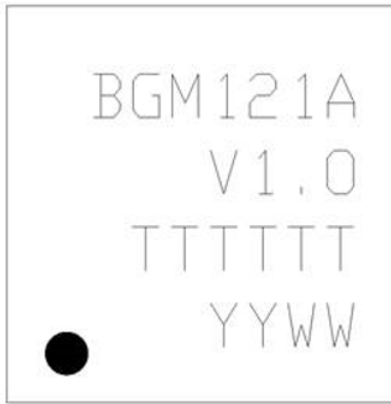
Figure 8.4. BGM121/BGM123 Package Marking
