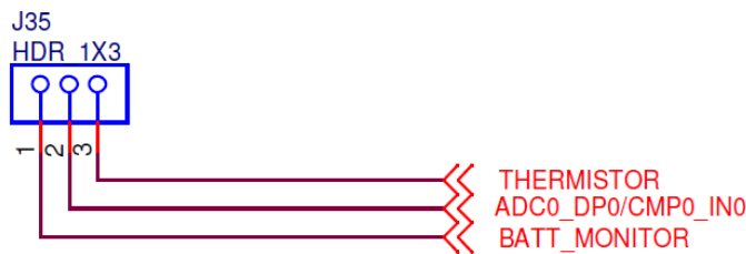
Figure 16: ADC0_DP0 selection jumper.
