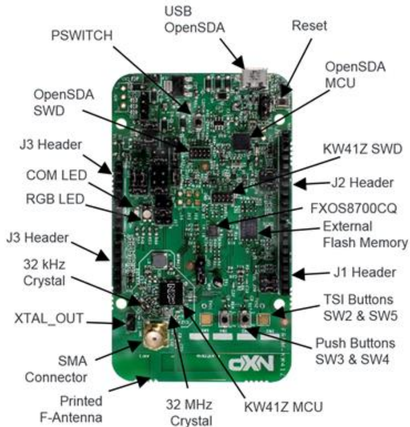
Figure 3: FRDM-KW41Z component placement.
