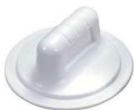
46006 Plastic knob with recess on sides of grip Material: ABS Diameter: 63 mm Height: 29 mm
