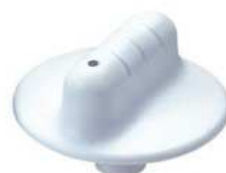
46005 Plastic knob, molded part only Material: PBT Diameter: 51 mm Height: 20 mm
