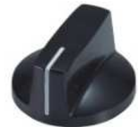
46117 Plastic knob with paint filled indicator line on top and side, glossy finish, fluted grip Material: ABS Diameter: 27.3 mm Height: 15.5 mm Shaft hole: D Type, 6 x 4.5 mm
