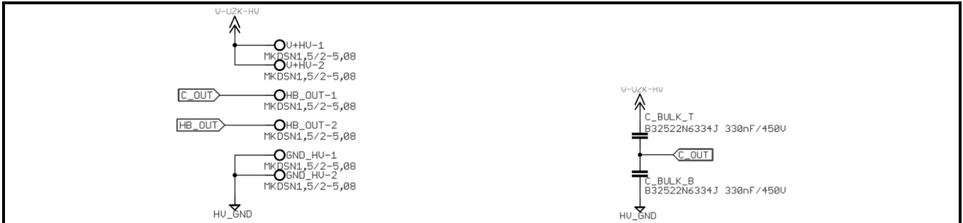
Figure 4-1: HV supply input and DC-Link capacitors
