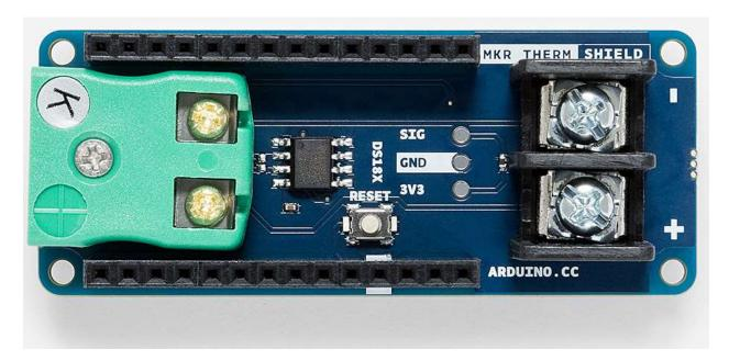
Thermocouples are based on the thermoelectric properties of a junction between two different metals and are capable of measuring with good precision ranges from -270 to +1372 Celsius (K type) that are far beyond any digital sensors or NTC/PTC (thermistor) range. A typical application of thermocouples is in boilers, soldering stations and coolers. Also good quality 3D printers rely on thermocouples to measure the extruder temperature.
