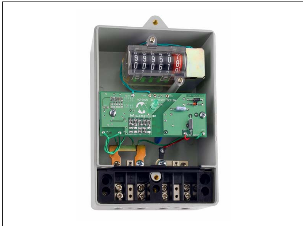
FIGURE 2-2: Photograph of Complete, Stand-Alone MCP3905 Energy Meter.
