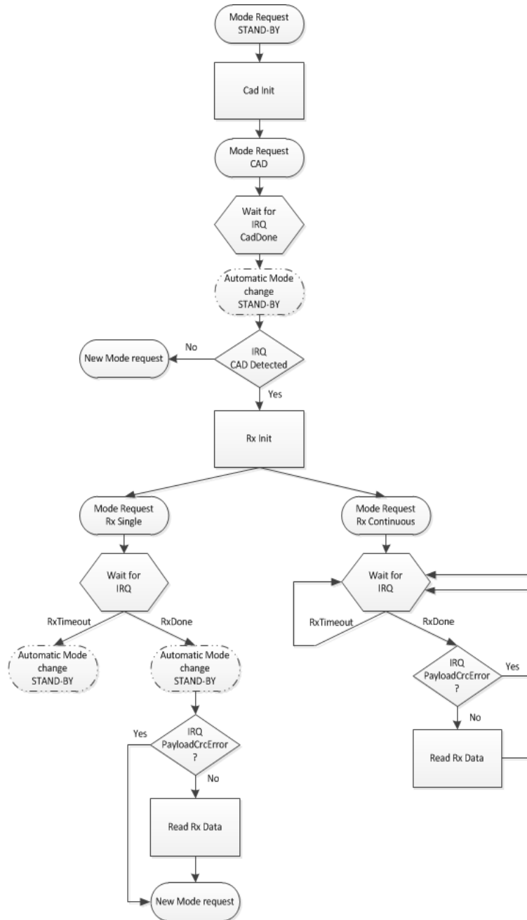
Figure 10. LoRa™ CAD flow
