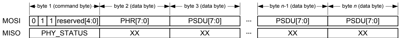
Figure 6-8. Packet Structure - Frame Write Access.
