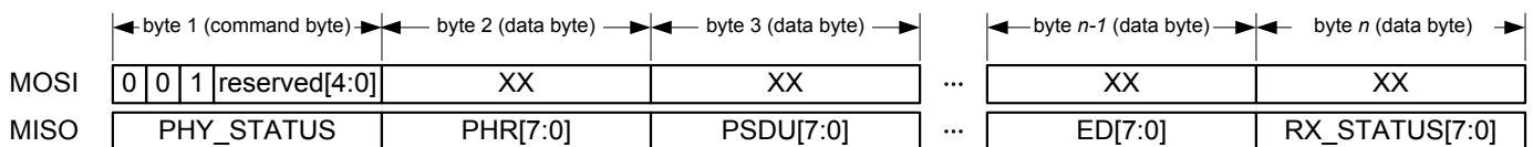
Figure 6-7. Packet Structure - Frame Read Access.
