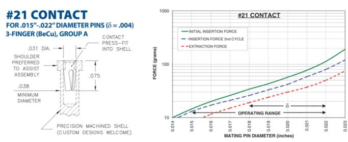
The insertion / extraction force characteristics above were derived using a 30 microinch gold-plated contact and polished steel gauge pins having a bullet-shaped tip.
