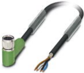
Sensor/Actuator cable, 4-position, PUR halogen-free, black-gray RAL 7021, shielded, free cable end, on Socket angled M8, Cable length: 3 m
