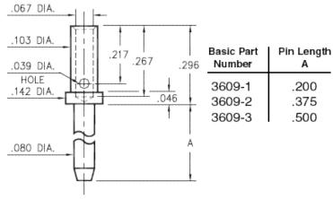
**Description:** 3609 - Wire Crimp Pin Packaging: Packaged in Bulk
