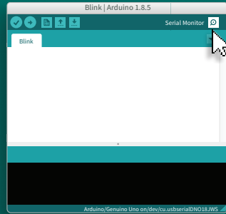
Serial Monitor button in the upper-right of the Arduino IDE.
