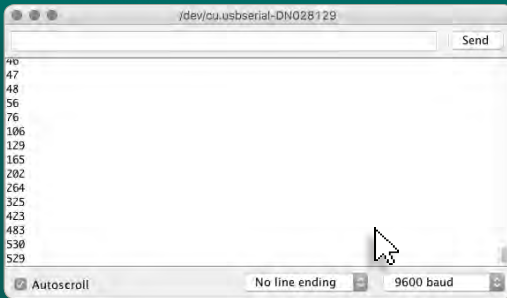
Serial Monitor printout and baud-rate menu.
