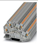
Double-level terminal block, nom. voltage: 500 V, nominal current: 22 A, connection method: Push-in connection, 1st and 2nd level, Rated cross section: 2.5 mm², cross section: 0.14 mm² - 4 mm², mounting type: NS 35/7,5, NS 35/15, color: gray
