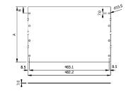
· Manufactured in aluminium, 3mm thick, clear anodised
