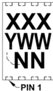
8-Lead DFN (2x3x0.9 mm)
