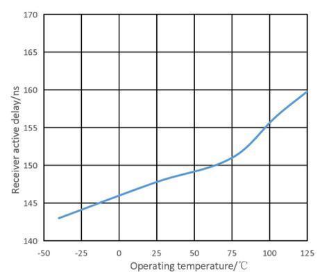
Figure 6. Receiver active delay VS Operating temperature
