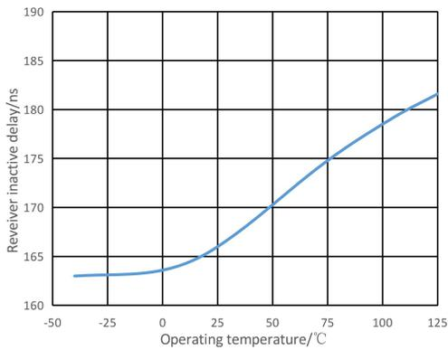
Figure 7. Receiver inactive delay VS Operating temperature
