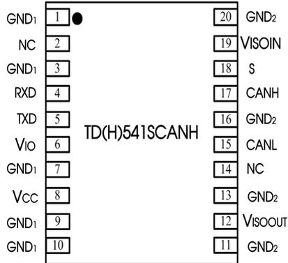
Note: All GND<sub>1</sub> pins are internally connected;
