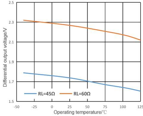
Figure 1. Drive differential output voltage dominant VS Temperature
