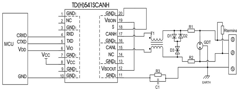
Figure 15. Port protection circuit for harsh environments
