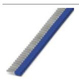
Taped ferrules, 0.75 mm², sleeve length: 8 mm, with plastic collars, according to DIN 46228-4, special color: blue according to NF C63-023, with function end for safe and convenient processing with the Crimphandy, 20 strips each with 50 sleeves per strip.
