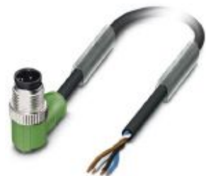
Sensor/actuator cable, 4-position, PUR halogen-free, black-gray RAL 7021, Plug angled M12, coding: A, on free cable end, cable length: 3 m
