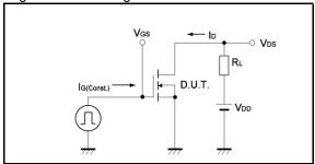
Fig.2-1 Switching Characteristics Measurement Circuit
