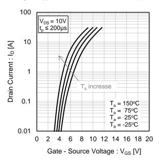
Fig.12 Typical Transfer Characteristics (II)
