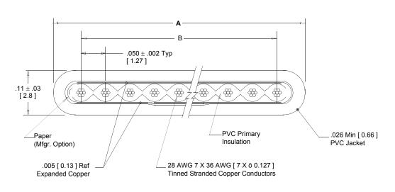
Note: Red marking on edge of primary cable designates wire #1.
