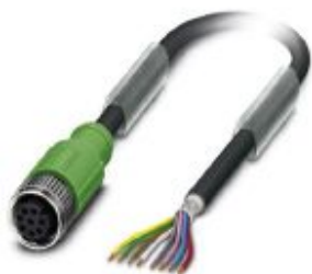
Sensor/actuator cable, 8-position, PUR halogen-free, black-gray RAL 7021, shielded, free cable end, on Socket straight M12, coding: A, cable length: 5 m
