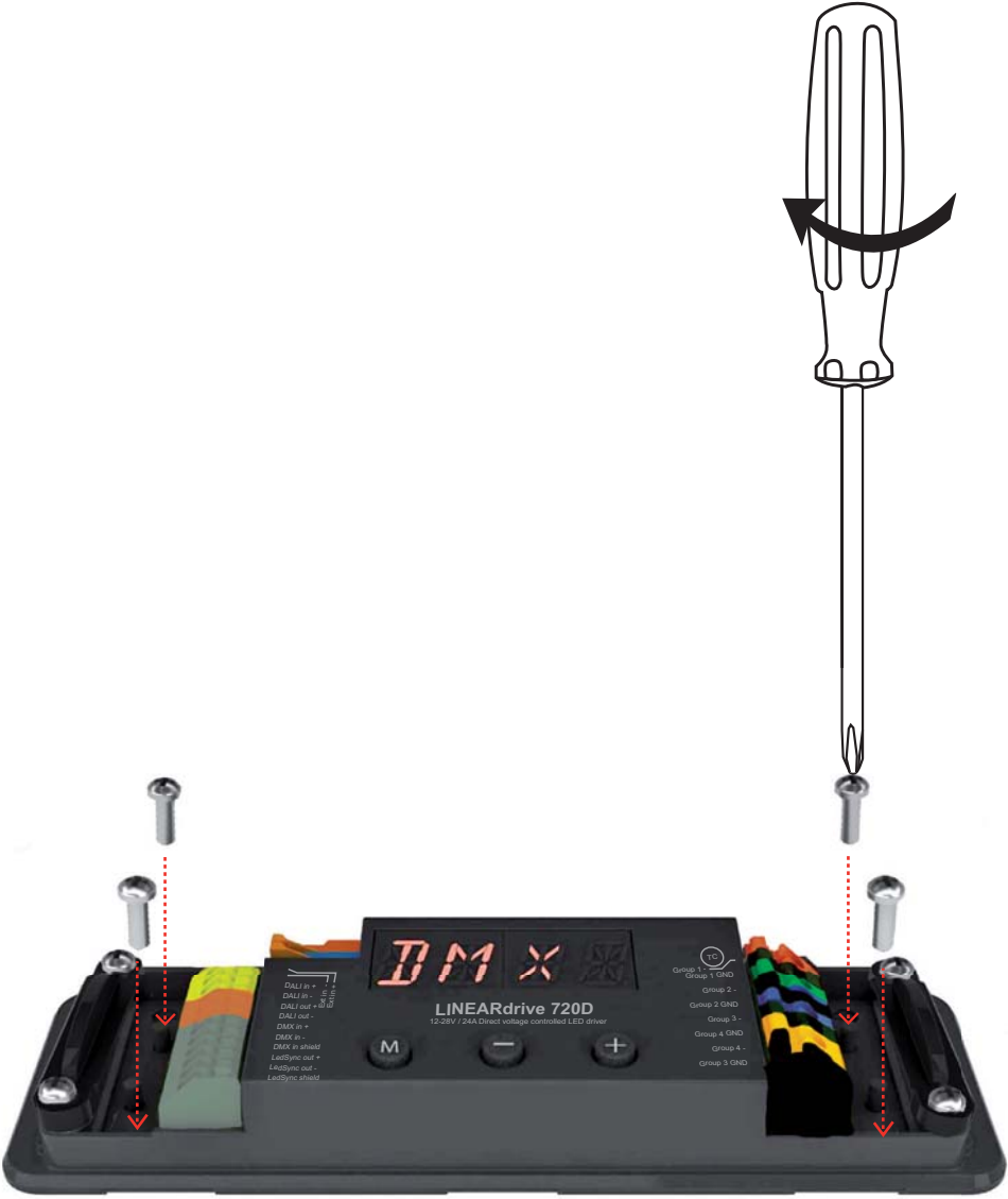
Figure 2.3: Fastening the mounting screws
