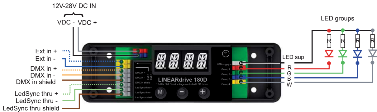
Figure 3.3: LINEARdrive Display 180 wiring diagram
