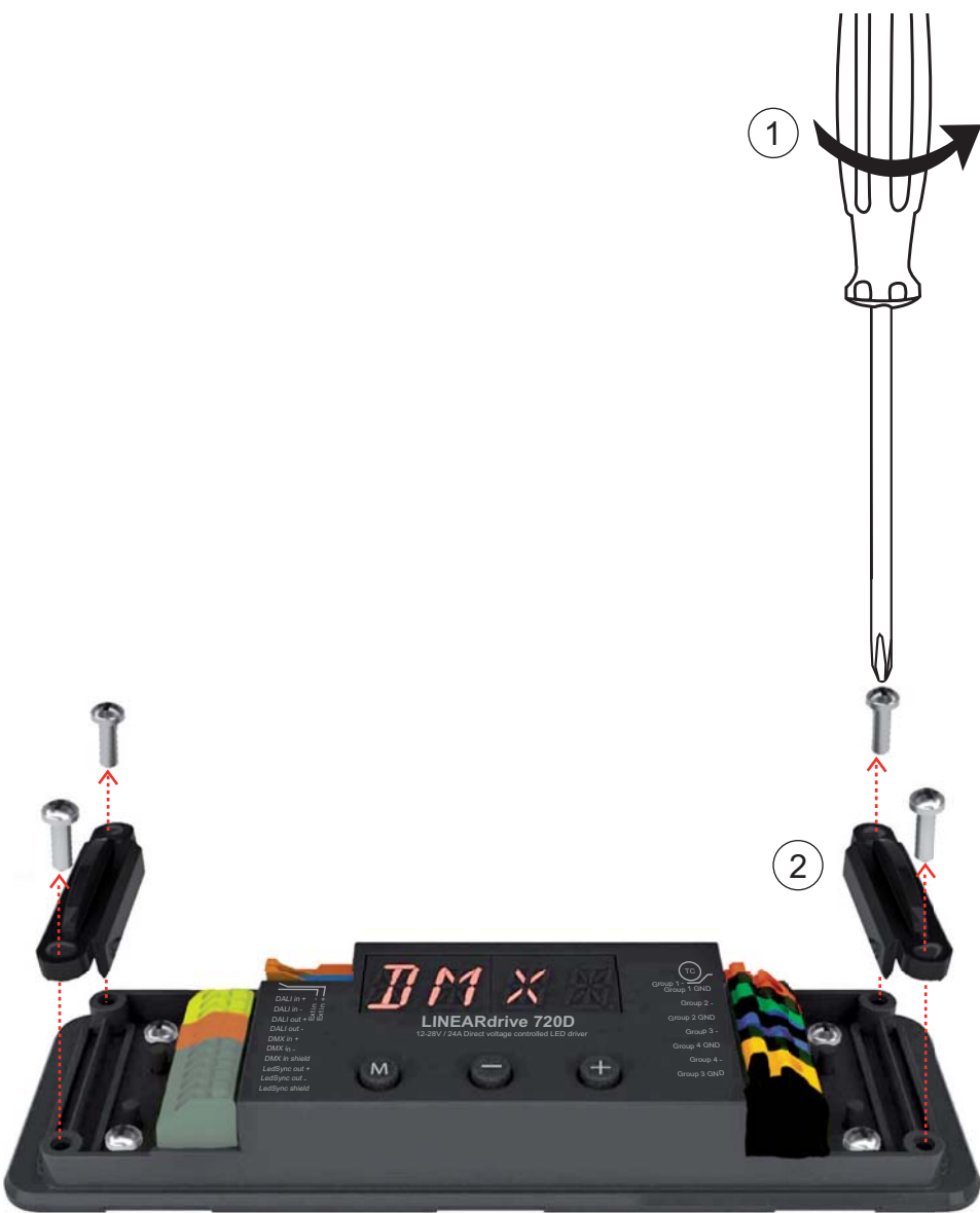
Figure 3.1: Removing the strain reliefs
