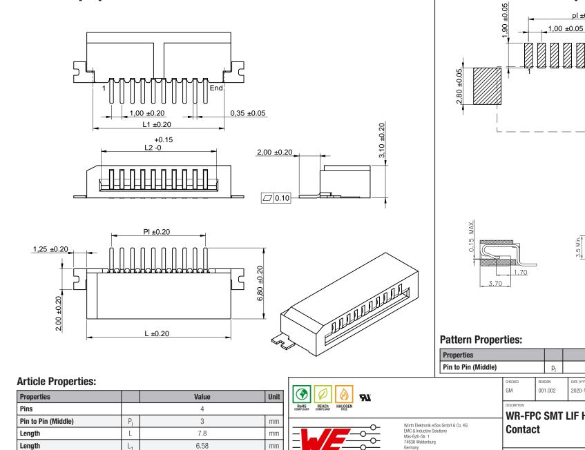
Unit Value 3 mm DATE (YYYY-MM-DD) GENERAL TOLERANCE PROJECTION METHOD 70 2020-10-29 DIN ISO 2768-1m **WR-FPC SMT LIF Horizontal Top** ORDER CODE 686104188622 SIZE/TYPE STATUS Tel. +49 (0) 79 42 945 - 0 BUSINESS UNIT PAGE 5.05 mm L<sub>2</sub> www.we-online.com WÜRTH ELEKTRONIK 1.00 mm eiCan Valid 1/7 eiSos@we-online.com
