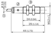
1 Connection 2 Indication LED 3 Fastening nuts (2x); width across 17, metal
