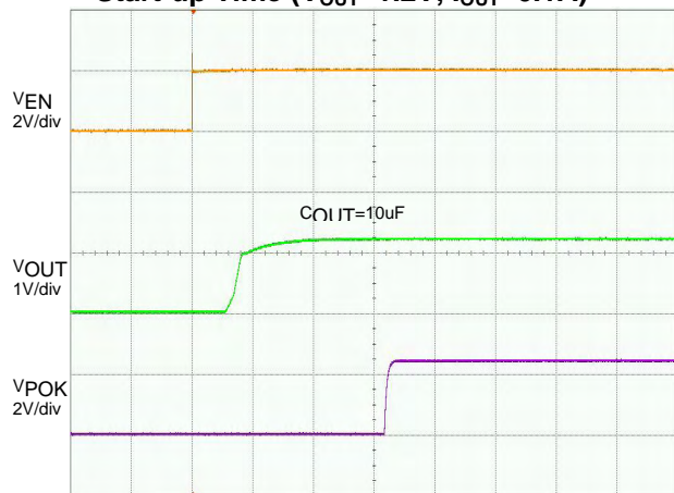
Start-up Time ( V_{OUT}=1.2V , I_{OUT}=0.1A )
