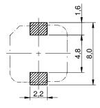
no sensitive traces underneath the component
