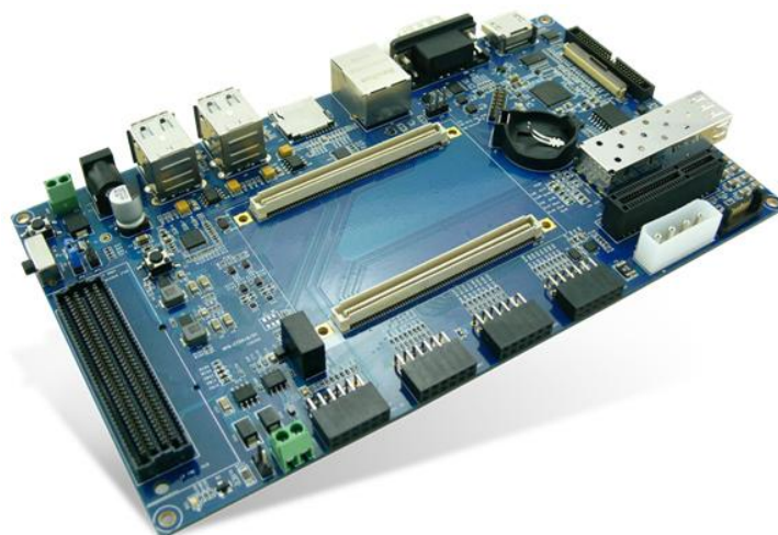
Figure 1-6 MYD-C7Z010/20-V2 Base Board for MYC-C7Z010/20-V2 CPU Module
