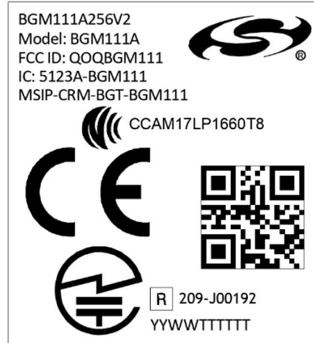
Figure 8.3. BGM111 Package Marking
