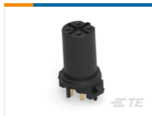
TE Part #494562-E M12 FEMALE, B CODE, 5P, 17MM THR
