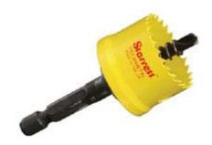
These tools have been engineered to maximize the utility of a handheld cordless drill. A constant pitch set of eight teeth per inch and durable bi-metal construction deliver vibration-free cutting action and extend the service time of battery operated tools. Smoothcut Cordless saws are an effective choice for most materials, including mild steel sheet, plasterboard, wood and thin non-metallics.
