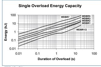
Mounted on a 0.53°C/W heatsink with 5m/s forced air cooling, air temperature 25°C. ΔR ≤ 5%.
