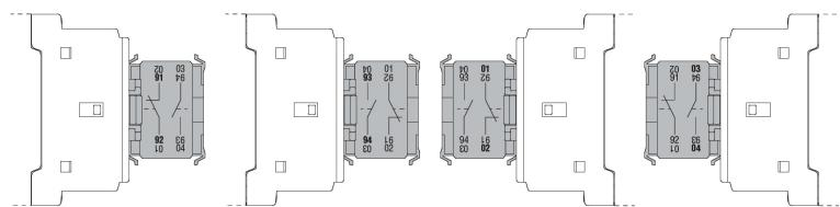
The termination of the G218 auxiliary contact has more than one numbering due to the fact that the block can assume various mounting positions. See the numbering in boldface for a correct interpretation.
