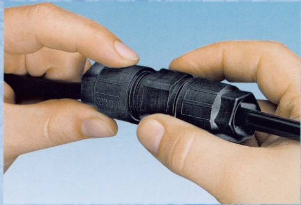
4. Place the union nut on the contact carrier and tighten with the necessary torque (5 Nm).
