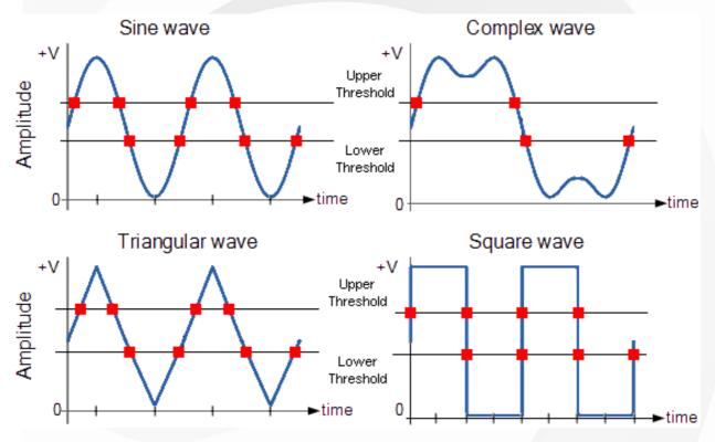
The Threshold upper and lower voltages can be set in the software
