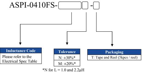
\*N for L = 1.0 and 2.2 $\mu$ H \*M for L = 2.2 ~ 47 $\mu$ H
