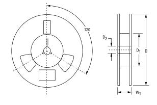
Devices are packed in accordance with EIA standard RS-481-A and specifications shown here.
