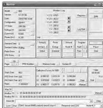
MultiView software will assist you in logging and downloading the electrical parameters captured with the M850-LTHN-RS-PO.
