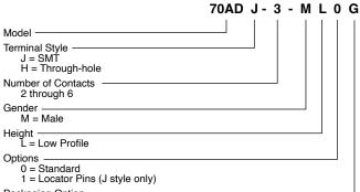
Packaging Option \_\_\_\_\_ = Tube (120/N pcs. or 120 contacts per tube)
