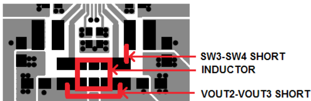
Figure 6. Combined 3A Regulator Inductor Placement and Connections
