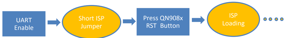
Fig 11. ISP download operation flow
