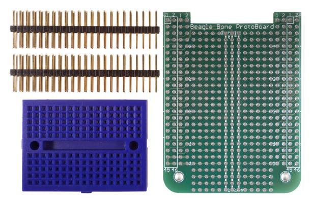
BeagleBone Through Hole Prototyping Cape(With Headers and Breadboard)
