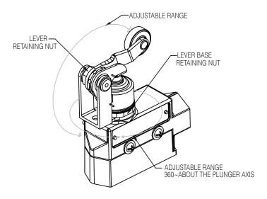
The lever can be adjusted in two ways. The following process details how to perform the adjustments.
