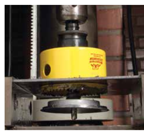
After the hole has been drilled, the core can clearly be seen at the end of the pilot drill.
