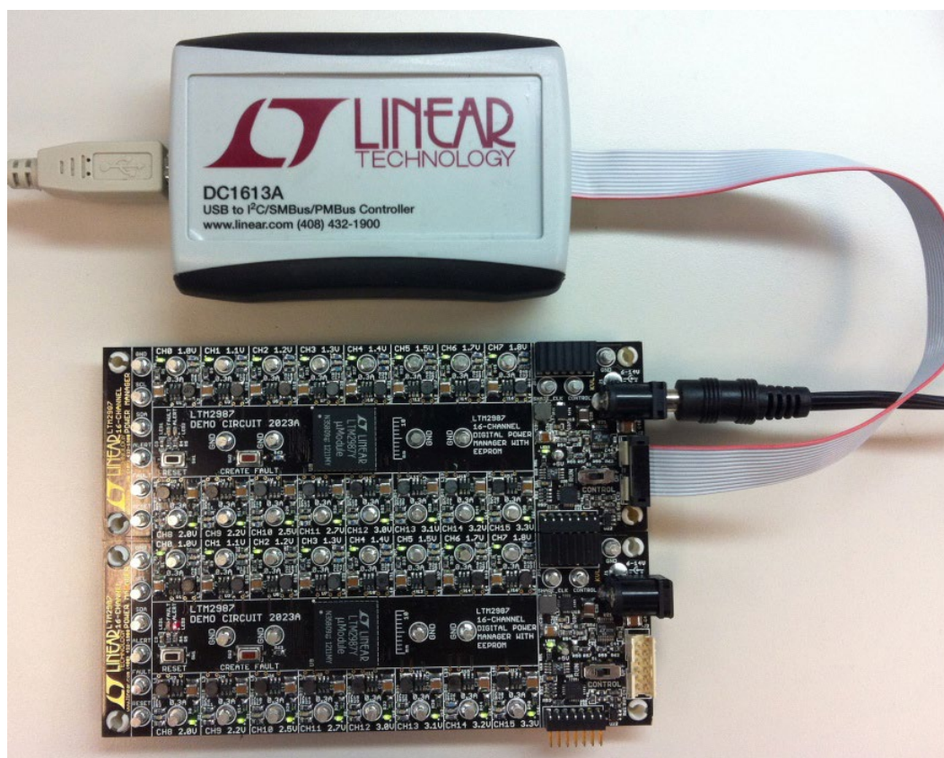
Figure 12. Array of Multiple DC2023A Demo Boards
