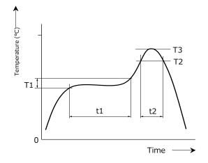
• Pb free solder recommended temperature profile Voltage Step-up Coils
