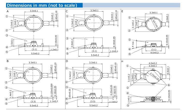
Part Name: ①Core ②Terminal ③Ring ④Coil ⑤Terminal board ⑥Adhesive
