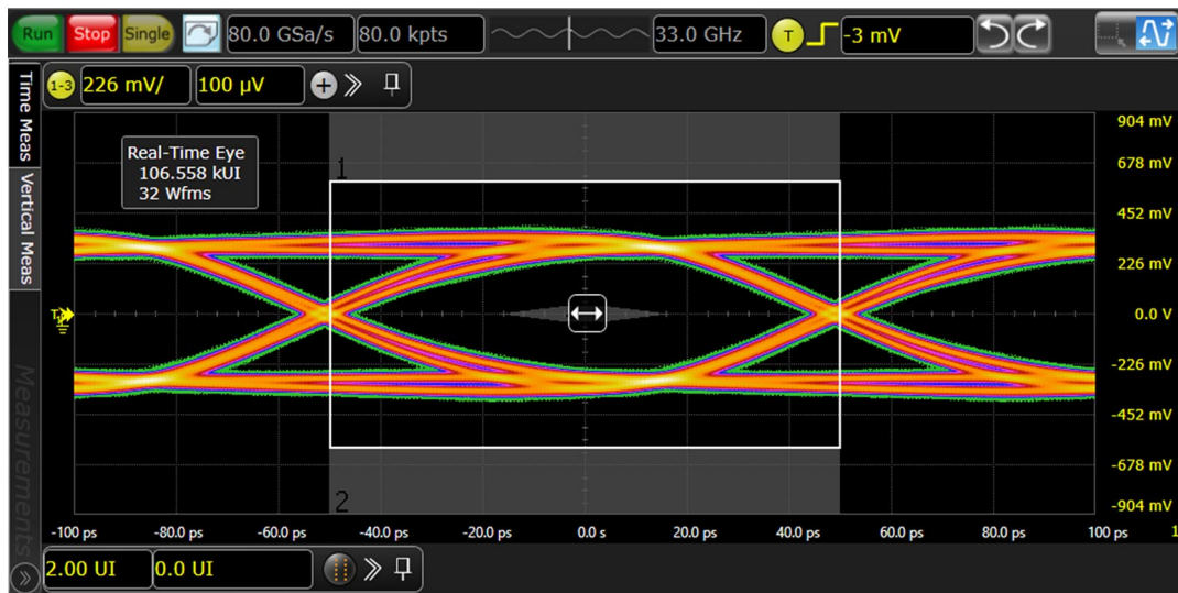
Fig. 8. USB 3.2 eye diagram, PCB with device; typical values
