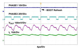
Figure 24. Boost Mode Waveforms, V<sub>IN</sub> = 9V, I<sub>OUT</sub> = 10A, CCM Mode
