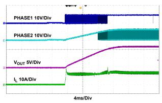
Figure 36. Start-Up Waveform,  $V_{IN} = 9V I_O = 10A$  CCM
