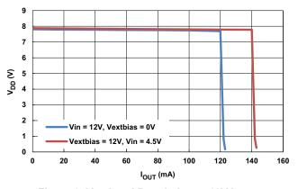
Figure 9.  $V_{DD}$  Load Regulation at 12V Input
