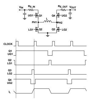
Figure 50. Buck-Boost Mode Equivalent Circuit and Operation Waveforms
