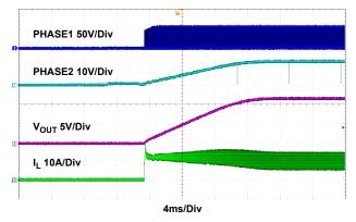
Figure 37. Start-Up Waveform,  $V_{IN}$  = 12V  $I_{O}$  = 10A, CCM
