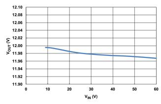
Figure 23. CCM Line Regulation at 10A Load +25°C
