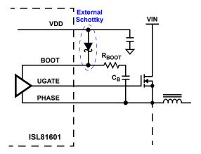
Figure 55. Upper Gate Driver Circuit
