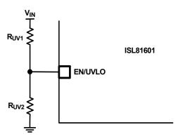
Figure 42. V<sub>IN</sub> Undervoltage Protection
