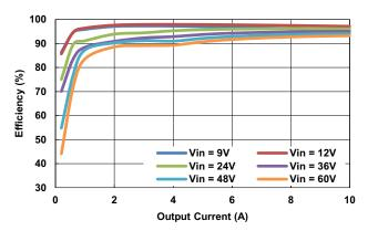
Figure 3. Efficiency ( $V_{OUT}$  = 12V, DE Mode)
