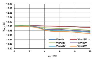
Figure 22. CCM Load Regulation at +25°C
