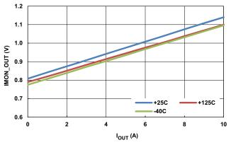
Figure 19. Output Current I $_{OUT}$  (DC) vs IMON\_OUT Pin Voltage, R $_{S\_OUT}$  =  $4m\Omega$ , R $_{IM\_OUT}$  = 40.2k
