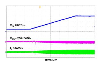
Figure 34. Line Transient,  $V_{IN}$  = 9V-60V, 1V/ms,  $I_{OUT}$  = 0A
