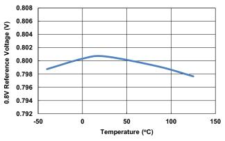
Figure 15. 0.8V Reference Voltage vs Temperature
