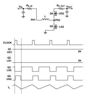
Figure 49. Boost Mode Equivalent Circuit and Operation Waveforms
