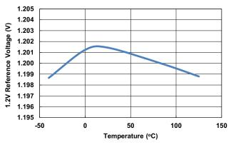
Figure 16. 1.2V Reference Voltage vs Temperature
