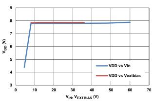
Figure 10. V<sub>DD</sub> Line Regulation at 20mA Load
