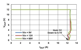
Figure 40. Constant Voltage (CV) and Constant Current (CC) Operation
