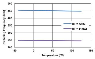
Figure 13. Switching Frequency vs Temperature
