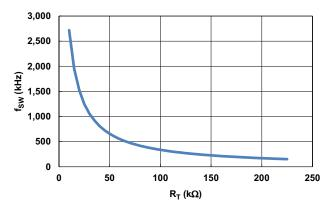
Figure 51. R<sub>T</sub> vs Switching Frequency f<sub>SW</sub>
