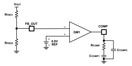
Figure 43. Output Voltage Regulator
