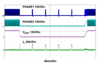
Figure 39. OCP Response, Output Short-Circuited from No Load to Ground and Released, CCM Mode,  $V_{\text{IN}}$  = 12V
