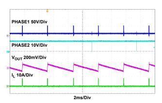
Figure 30. Burst Mode Waveforms,  $V_{IN}$  = 60V,  $I_{OUT}$  = 0.1A
