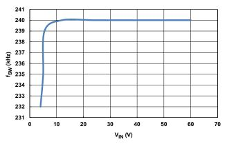
Figure 14. Switching Frequency vs  $V_{IN}$ ,  $R_T = 144k$
