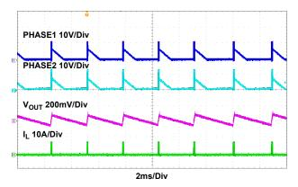
Figure 29. Burst Mode Waveforms, V<sub>IN</sub> = 12V, I<sub>OUT</sub> = 0.1A
