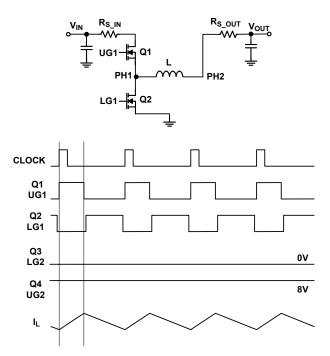
Figure 48. Buck Mode Equivalent Circuit and Operation Waveforms
