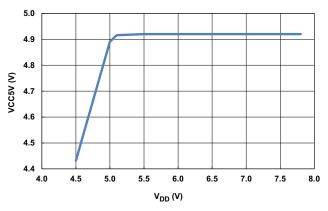
Figure 12. V<sub>CC5V</sub> Line Regulation at 20mA Load
