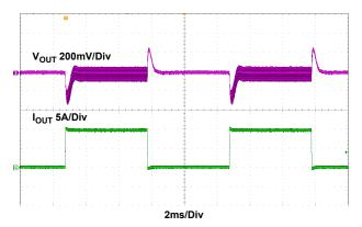
Figure 31. Load Transient,  $V_{IN}$  = 9V,  $I_{OUT}$  = 0A to 10A, 2.5A/µs, CCM
