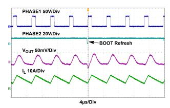
Figure 26. Buck Mode Waveforms, V<sub>IN</sub> = 60V, I<sub>OUT</sub> = 10A, CCM Mode
