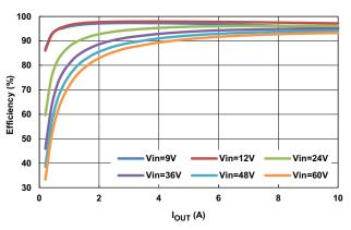
Figure 20. CCM Mode Efficiency
