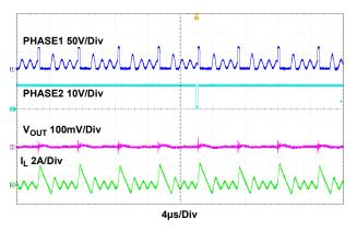
Figure 27. DE Mode Waveforms,  $V_{IN}$  = 60V,  $I_{OUT}$  = 0.2A
