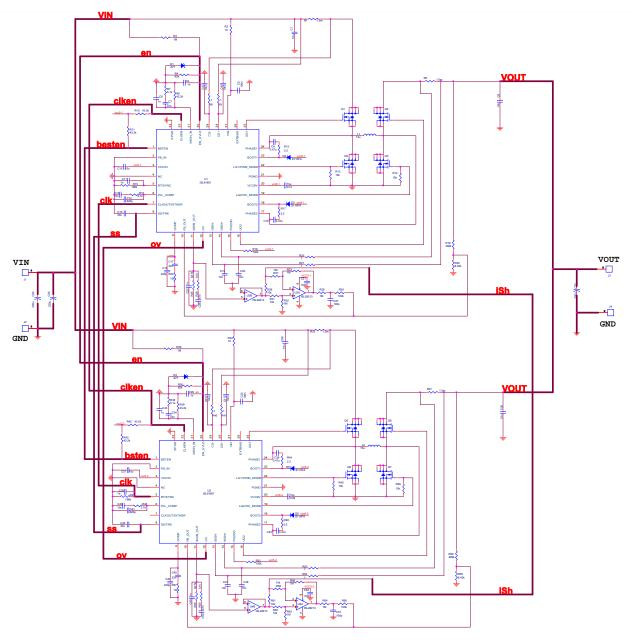
Figure 54. ISL81601DEMO1Z Current Sharing Circuit
