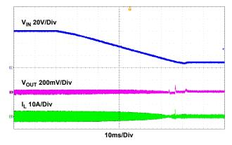
Figure 35. Line Transient,  $V_{IN} = 60V-9V$ , 1V/ms,  $I_{OUT} = 0A$
