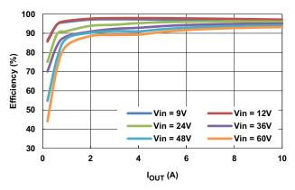
Figure 21. DE Mode Efficiency
