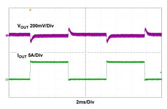
Figure 33. Load Transient,  $V_{IN}$  = 60V  $I_{OUT}$  = 0A to 10A, 2.5A/µs, CCM
