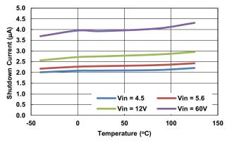
Figure 7. Shutdown Current vs Temperature
