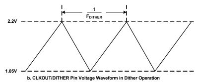
Figure 53. Frequency Dithering Operation
