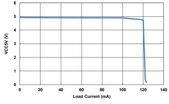
Figure 11.  $V_{CC5V}$  Load Regulation at  $12V_{IN}$
