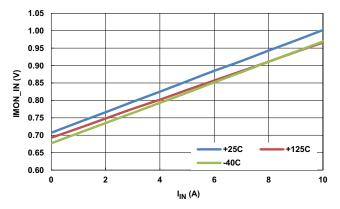
Figure 18. Input Current I<sub>IN</sub> (DC) vs IMON\_IN Pin Voltage,  $R_{S\ IN}$  = 4m $\Omega$ ,  $R_{IM\ IN}$  = 36k
