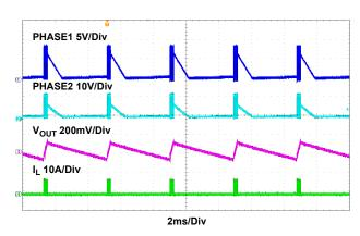
Figure 28. Burst Mode Waveforms,  $V_{IN}$  = 9V,  $I_{OUT}$  = 0.1A
