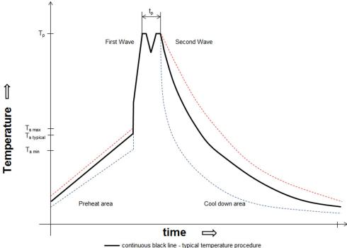
continuous black line - typical temperature procedure ------ interrupted blue line - min temperature procedure ------ interrupted red line - max temperature procedure
