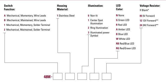
\* Current limiting resistor is required to limit LED forward current to 20 mA (not included).
