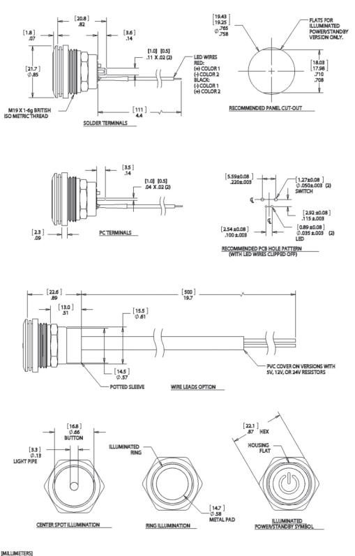
ELECTRICAL SPECIFICATIONS Current rating (resistive): 250mA @ 12VDC, 100K Cycles 150mA @ 28VDC, 150K Cycles (Momentary)
